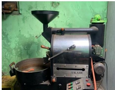
Gambar 3.2. Mesin Roasting di UMKM (centrifugal roaster)
